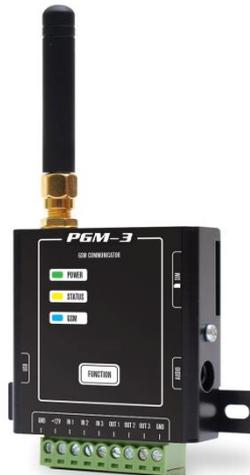
Pacific GSM company has expanded its range of GSM communicators in a micro version – in robust metal enclosure with 3 inputs and 3 outputs, audio input and output. We have designed a multifunctional communication device that offers a simple yet flexible method of transmitting critical data via the GSM network.
